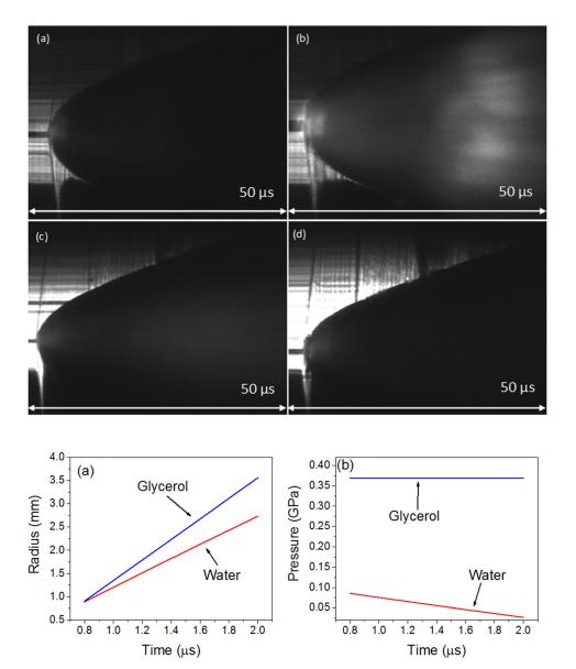
FIG. 13. Typical laser backlit streak images with a streak of  $2.5 \,\mu$ s/mm. Explosion of (a) Cu and (b) Al wires in water and (c) Cu and (d) Al wires in glycerol.
