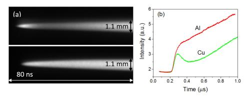
FIG. 8. Typical streak images of the self-light emission from the exploding Cu (a) and Al (b) wires in water and their intensity integrated along the vertical axis versus time. These streak (50 ns/mm) images were obtained with a low pass optical filter of 700 nm.
