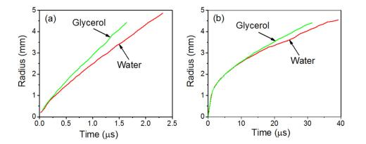
FIG. 5. Typical radial trajectories of the generated SW (a) and expanding Cu wire (b) versus time in water and glycerol.
