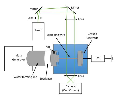
FIG. 1. Experimental setup. CVR is the current view resistor, and VD is the output from the high voltage electrode connected to the Tektronix high-voltage divider.
