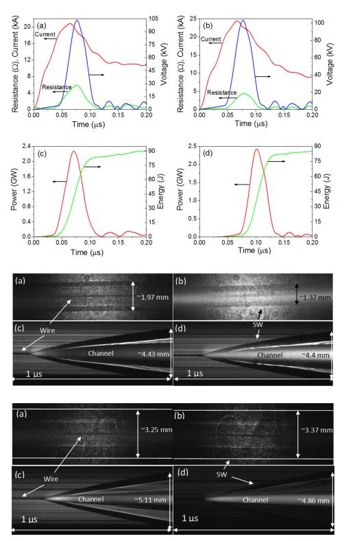
FIG. 2. Waveforms of the discharge current, resistive voltage, and wire resistance in the case of (a) Cu wire and (b) Al wire ns-timescale explosions in water. Power and energy temporal evolution for (c) Cu wire and (d) Al wire explosions.
