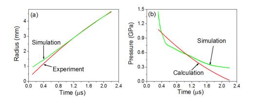
FIG. 6. (a) Measured and simulated position of the SW in water. (b) Calculated and simulated pressure behind the SW front.
