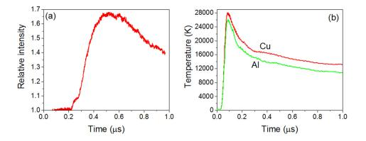
emission intensities obtained in the case of Al and Cu wires' electrical explosions in water; (b) simulated temperature at the surface of the Al and Cu wires during the explosion.
