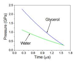
FIG. 7. Pressure calculations behind the front of the SW generated by a Cu wire electrical explosion in water and glycerol.
