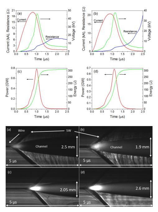
FIG. 11. Waveforms of discharge current, resistive voltage, and wire resistance in the case of (a) Cu wire and (b) Al wire electrical underwater explosions. Power and energy temporal evolution for (c) Cu and (d) Al wire explosions.
