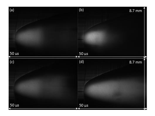
FIG. 10. Typical laser backlit streak images (2.5 µs/mm) of exploding Cu (a) and Al (b) wires in water and Cu (c) and Al (d) wires in glycerol.
