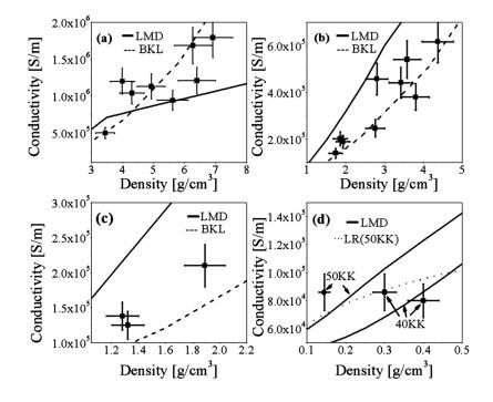
FIG. 5. Electrical conductivity of Cu for temperatures of (a) 10 KK, (b) 20 KK, (c) 30 KK, and (d) 40–50 KK. Symbols denote experimental results, the solid line denotes LMD model, the dashed line denotes BKL model, and the dotted line denotes LR model.
