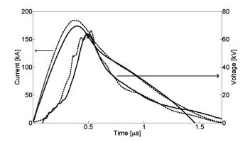
FIG. 3. Experimental and simulated current and voltage waveforms of exploding 0.5 mm diameter Al wire. Solid lines denote experimental data and dashed lines denote simulated data.
