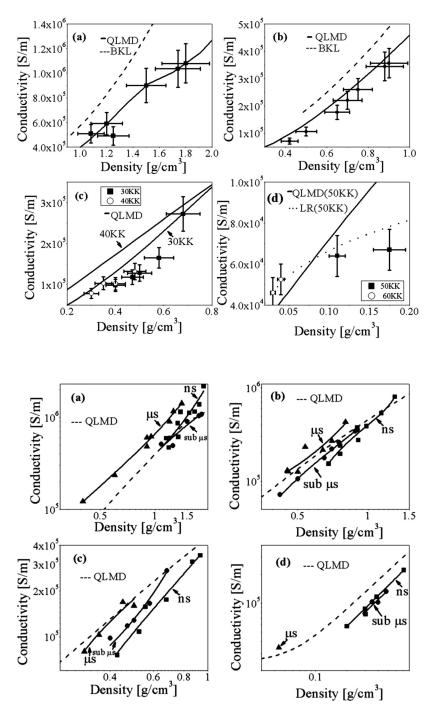
FIG. 6. Electrical conductivity of Al for temperatures of (a) 10 KK, (b) 20 KK, (c) 30–40 KK, and (d) 50–60 KK. Symbols denote experimental results, the solid line denotes QLMD model, the dashed line denotes BKL model, and the dotted line denotes LR model.
