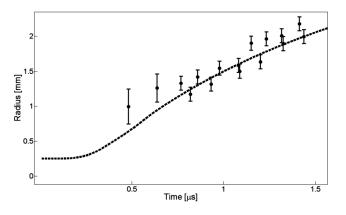
FIG. 4. Experimental and simulated radial wire boundaries for the case of exploding 0.5 mm diameter Al wire. Symbols denote experimental data and the dashed line denotes simulated data.
