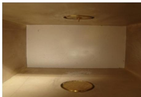
FIG. 9. Cone electrodes used to initiate the plasma discharge in the Magic-tee side-arm.
