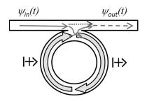
Fig. 2. Auxiliary problem. Phase matched coupling between waveguide and waveguide modes. Notation is the same as in Fig. 1.
