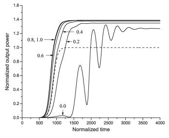
Fig. 4. Same as in Fig. 3. "Long" feedback loop,  $\theta \gg Q_{leak}/|q|$ .  $|Q_{diss}| = 15$ ,  $Q_{leak} = 20$ , q = 0.2, and  $\theta = 200$ .
