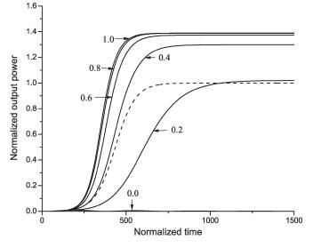
Fig. 3. Dependence of the normalized power on time. "Short" delay time  $\theta < Q_{leak}/|q|$ . Dashed line corresponds to q = 0. The curves are marked by corresponding  $\alpha/\pi$  values.  $|Q_{diss}| = 15$ ,  $Q_{leak} = 20$ , q = 0.2, and  $\theta = 70$ .
