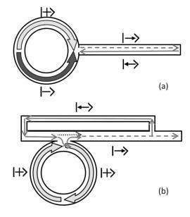
Fig. 1. Magnetron (ring resonator) and waveguide. (a) Clockwise  $|+\rangle$  and (light-gray bold arrow) and anti-clockwise  $|-\rangle$  (dark-gray bold arrow) propagating eigenmodes. Direct (dashed line) and reflected (solid line) waves in the waveguide. (b) Ring resonator side-coupled to a waveguide with a feedback loop.
